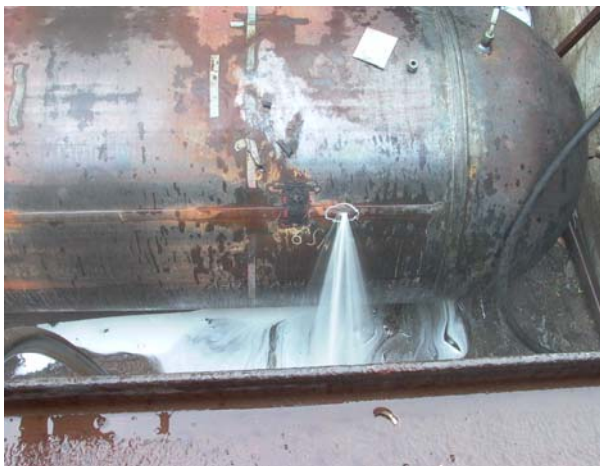
Fig. 8 Fatigue failure at corrosion pitting in long seam
