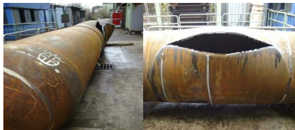
Fig. 9 Full scale fatigue-burst test
