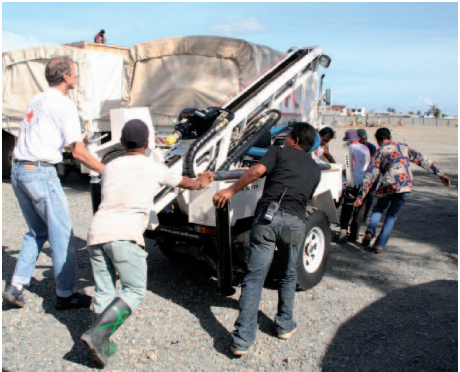
The Norwegian Red Cross team prepares the drilling rig for operation in Banda Aceh, Indonesia. The drilling rig, which can drill down to approximately 100 metres, is fitted on a trailer and pulled by a Red Cross land cruiser.
